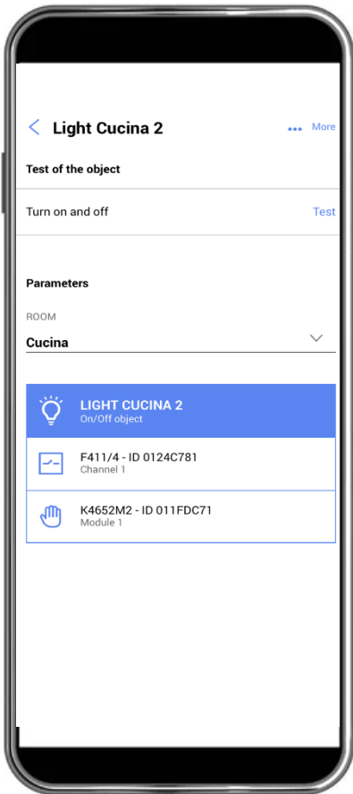
The app provides configuration information and the type of associated actuator.
