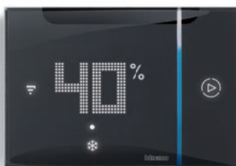
Display the set room temperature and humidity
