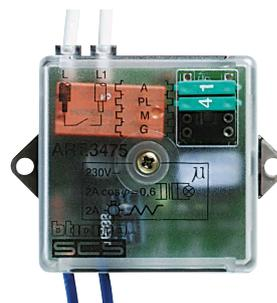
**Actuator, item 3476** with 1 relay for single loads: 2 A resistive or incandescence lamps, 2 A inductive for ferromagnetic transformers. Preset for connection with NO type control pushbutton.
