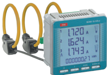
KIT NEMO 96 HDLe + Rogowski coils KIT ready for installation including 1 multifunction + 3 Rogowski coils 3 current ranges that can be selected on each KIT: 20...1000A, 60...3000A, 100...5000A
