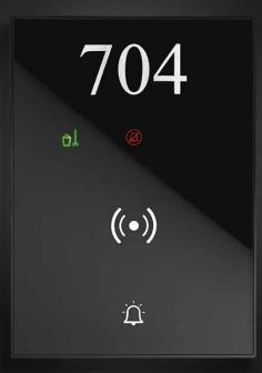
OUTSIDE THE DOOR INDICATOR + KEY CARD READER It includes the key card reader in RFID technology and the luminous notifications: (DND) Do Not Disturb, (MUR) Make Up Room indicator and touch pushbutton to activate the bell in the room. Possibility of customising the product with room number.
