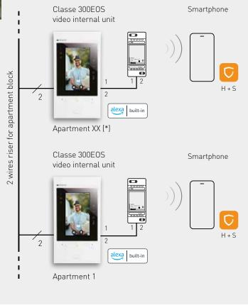
NOTE: for the sizing of multi-family systems refer to the General Installation Standards of the 2 Wires System Technical Guide.
