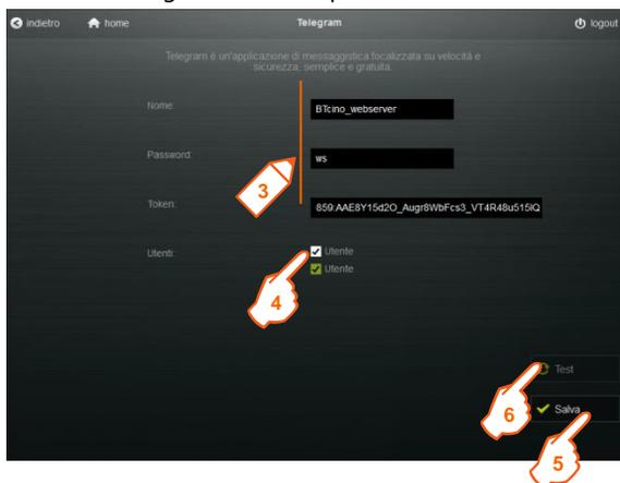
This screenshot shows the same Telegram configuration page as above, but with the fields filled in. Red callout boxes with numbers 3 through 6 point to specific elements: 3 points to the 'Nome' field containing 'BTicino\_webserver'; 4 points to the 'Utenti' section where both 'Utente' options are checked; 5 points to the 'Salva' button; and 6 points to the 'Test' button. The 'Password' field contains 'ws' and the 'Token' field contains '859AAE8Y15d2O\_Auqr8WbFcs3\_VT4R4Bu516Q'.
